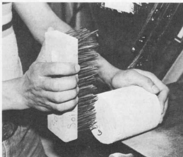
(c) Closeup view of brushing strokes applied to the end of a soil-cement durability test specimen.
