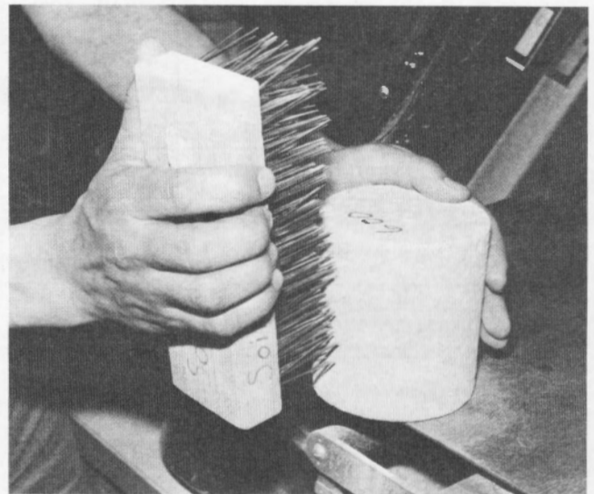
(b) Closeup view of downward vertical brushing strokes applied to the sides of a soil-cement durability test specimen.
