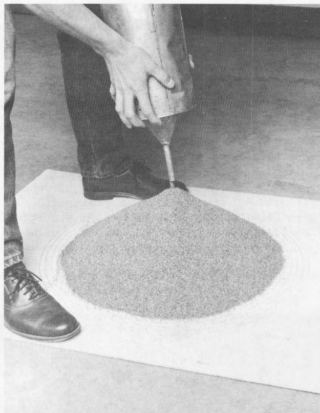
Figure 3. – Placement of soils of 3/8-inch maximum particle size while maintaining a 1-inch free fall height. The pouring device is a 6-inch-diameter by 12-inch-high cylinder with a 1/2-inch funnel.
