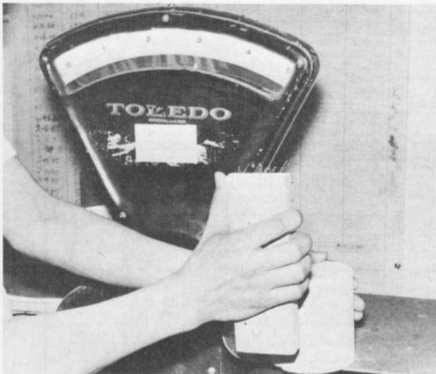
(a) Brush strokes applied to a soil-cement durability test specimen registering a 3 lbm on platform scale.
