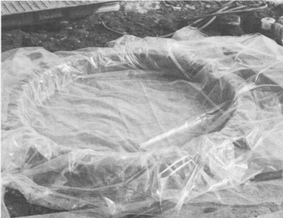
Figure 5. – Plastic liner placed in preparation for the initial volume determination.
