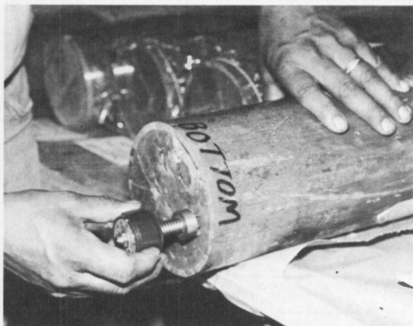
Figure 2. – Torvane used on the end of a tube-type sample.
