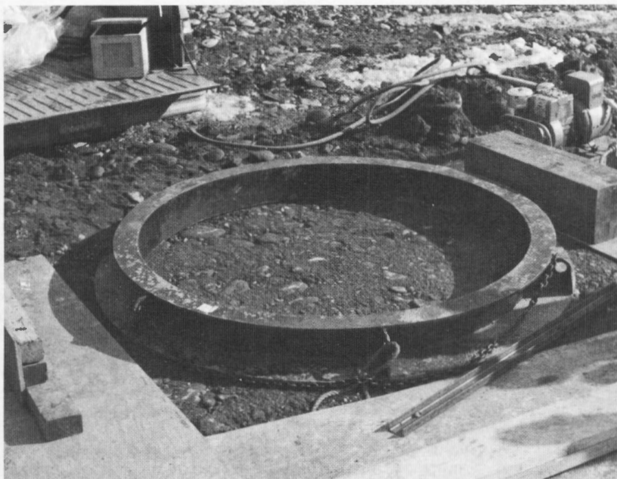
Figure 1. – A 6-foot-diameter metal ring for determining in-place unit weight.
