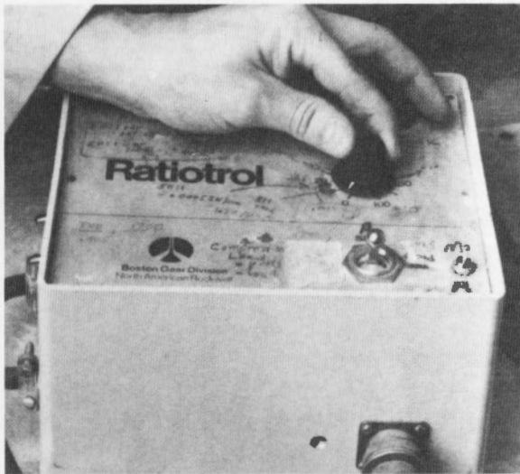
(b) Electronic control box for controlling the displacement rate.
