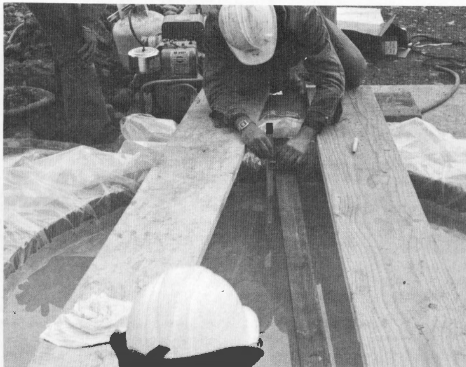
Figure 6. – Measuring the reference water level with carpenter's square.
