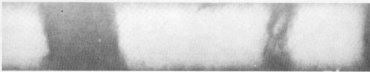
Figure 2. — X-ray radiograph showing void (dark area) and gouge zone in tube-type soil sample.
