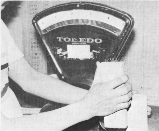
(a) Brush strokes applied to a soil-cement durability test specimen registering a 3-lbm on platform scale.
